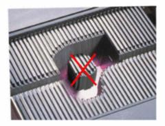
Center of beam cannot be shielded... using a single, "rapid arc" compromises must be made
